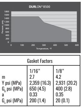
Fire Testing: Durlon® 8500 has successfully passed the API 6FB fire test [avg. temperature >650°C, 30 mins, 40 bar, 1 ml (inch/ min.) maximum allowable leakage].
