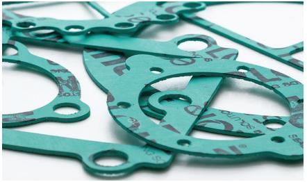
A high performance compressed gasket material for use in process industries including pulp & paper, food & beverage, pharmaceutical, hydrocarbon, chemical, refinery and general industry. Durlon<sup>®</sup> 8500 is suitable for oils, water, steam, new generation refrigerants, dilute acids & alkalis and many other liquids & gases and has passed the API 6FB Fire Test and conforms to FDA 21 CFR 177.2600 Rubber articles intended for repeated use.
