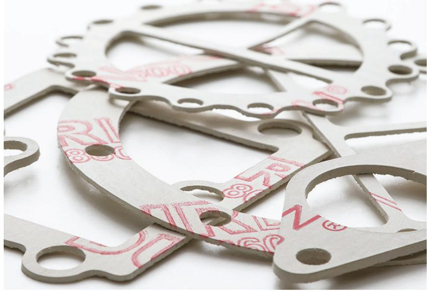
Durlon® 8600 is a quality compressed sheet gasket material for use in process industries including pulp & paper, power, petrochemical as well as general industry where a “white” gasket material is often required when working with food & beverage, pharmaceutical and plastics. Applications: water, steam, air, inert gases, alcohols, dilute acids and alkalis.
