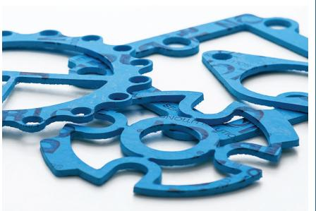
Durlon<sup>®</sup> 8700 is a high performance gasket material for use in processes requiring a neoprene (CR) bonded sheet. This product has excellent resistance to ozone, oils, non-aromatic solvents and many refrigerants. Durlon<sup>®</sup> 8700 has excellent hand and die cutting characteristics and has passed the MIL-G-24696B Navy Adhesion Test (366°F/48 hrs).
