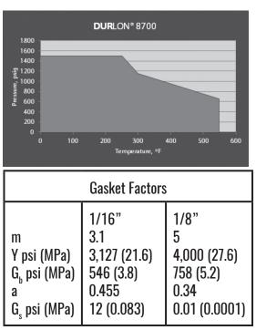
Anti-Stick Properties: Much effort has gone into improving the anti-stick release agents of all compressed Durlon® products. All Durlon® compressed gasket materials have passed the MIL-G-24696B Navy Adhesion Test (366°F/48hrs).
