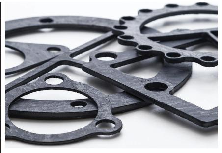
A premium grade material for service conditions to 496°C (925°F) and continuous operating temperatures of -73°C to 400°C (-100°F to 752°F). Durlon® 8900 is ideal for saturated and superheated steam, oil, dilute acids and alkalis, hydrocarbons, and solvents and has passed the extreme conditions of API 607 (6th edition) Fire Test with documented zero leakage.
