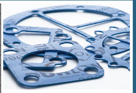
Durlon<sup>®</sup> 9002 is an adaptation of the original glass-filled formula to better meet extreme cryogenic demands. Durlon<sup>®</sup> 9002 has passed BAM certification for both gaseous and liquid oxygen tests up to 260°C (500°F) at 52 bar (754 psi) and LOX Mechanical Impact Sensitivity (ASTM G86 & ISO 21010), passing with zero reactions out of twenty tests (0/20) at a test reaction frequency of 0%.
