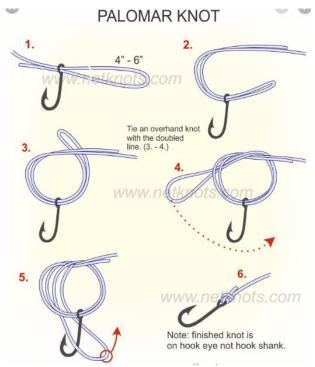
• The Palomar knot is used to tie fishing line to a hook, lure, or swivel. Easier to tie than the Clinch knot
