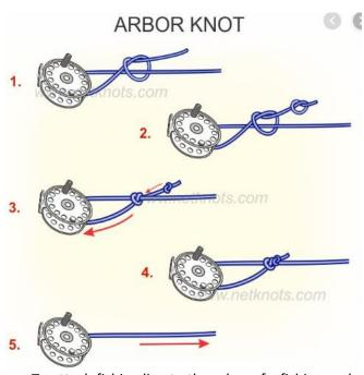
To attach fishing line to the arbor of a fishing reel.
