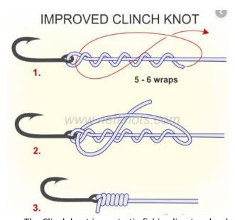
• The Clinch knot is use to tie fishing line to a hook, lure, or swivel. Do not use with heavy line.
