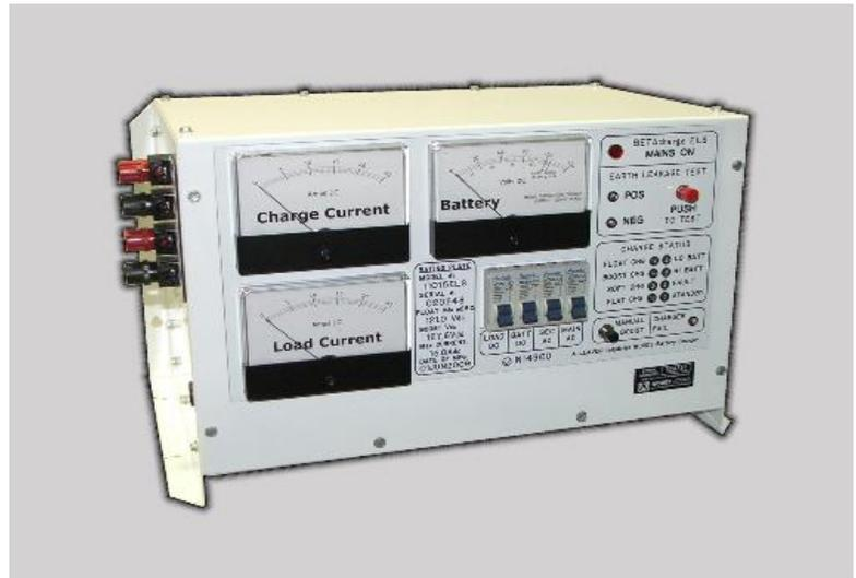
The WOODS BETAcharge II ELS is a sophisticated electronic multiple-taper charger for most types of batteries. It employs microprocessor-controlled SCR's to precisely regulate charging voltages and currents during all phases of charging. The BETAcharge II ELS successfully charges deeply discharged batteries and batteries which are loaded during charging.
