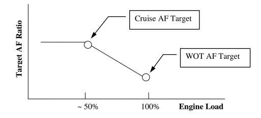
Just as the Cruise Air/Fuel target can be adjusted for fuel economy, the WOT Air/Fuel target can be adjusted for maximum power. It is quite possible that the engine can make more power at an air/fuel ratio that is leaner (higher number) than the preloaded WOT Air/Fuel target. Or it might prefer a richer (lower number) air/fuel ratio. This is less likely, but it all depends on the engine.
