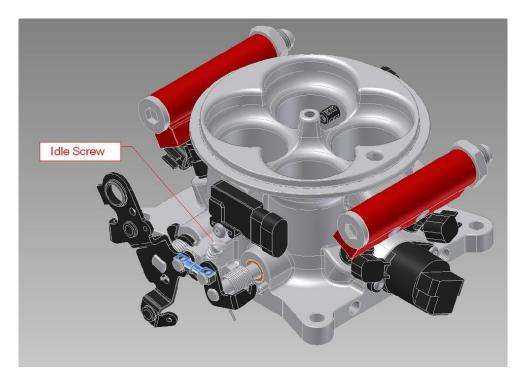
**13. TPS IDLE RE-CALIBRATION.** The throttle position sensor is connected to the throttle shaft. So adjusting the resting position of the throttle blades in the previous step may have changed the voltage the ECU is receiving from the TPS. To account for this, you will again be asked to leave the throttle at the idle/closed position and let the ECU capture that voltage.
