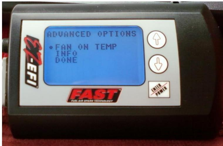
7. **FAN ON TEMP.** This sets the engine temperature that will activate the Fan output. When the temperature exceeds this limit, the Fan output wire switches to ground to control a relay. Do **NOT** wire the Fan output directly to a fan. Once the temperature has dropped 20\*, the Fan output will be deactivated.
