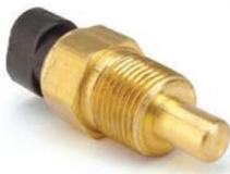
The Coolant Temperature Sensor monitors engine coolant temperature. It is typically installed in an existing mounting hole on the top of the intake manifold. The sensor has 3/8" NPT threads. The supplied adapter may be required to install the sensor in some manifolds with 1/2" NPT threads. The engine block or cylinder head may have a provision for mounting a coolant temperature sensor. Just be
