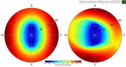
Above, stereoplot showing required mud weights to keep a borehole stable for an isostropic (left) and anisotropic (i.e, planes of weakness, right) cases. To the right, an example of splintery cavings indicative of shear failure at the wellbore wall (from Zhang, and Yin, 2017 licesenced under CC BY 4.0).
