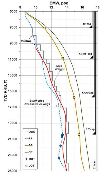
Fracture Gradient Prediction. We help you mitigate drilling induced losses by predicting changes in fracture gradient magnitude with depth and defining the maximum allowable bottom hole pressure to avoid fracturing the formation. We provide accurate predictions for scenarios of particularly low fracture gradient where there is a high risk of lost circulation. These scenarios include overpressured deepwater wells and well paths that intersect faults or depleted reservoirs.
