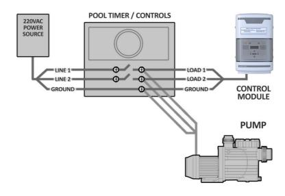
In some parts of the United States and Canada, the Control Unit must be connected to a circuit protected by a Class A ground fault interrupter (GFI). Check local codes before connecting.
