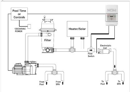
There are three main Parts to the CFSC system: The Control Unit, the Electrolytic Cell, and the Flow Switch.
