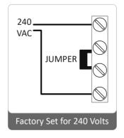
This set of terminal screws can be located inside of the Control Unit, and accessed by removing the four screws from the Control Unit's aluminum base. The factory voltage setting is the 240V configuration, with a jumper clip inserted between the second and third terminals. The Control Unit can be made to accept 110V by reconfiguring the jumper clips as shown above left, with two jumper clips instead connecting the first and second terminals, and the third and fourth terminals.
