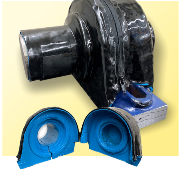
Above: Enviropeel Bearing Shield zipped on to substrate and open to show inside layer of Enviropeel.
