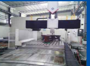
数控定梁龙门五面加工中心 CNC fixed beam gantry five face machining center
