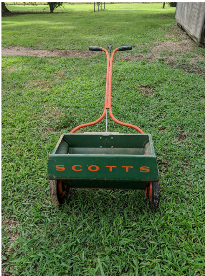
Figure 4. Although a drop spreader like this one can be used, it is often more time consuming and can be more difficult to get a uniform stand.
