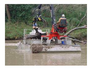
d). Clearing trees from the banks of a creek or bayou are painless when using the hydraulic driven chainsaw with rotating grapple.
