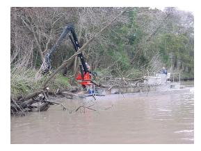
e). Loading the hopper of the barge only takes minutes when dealing with average size trees (up to 18 inches) then it's time to head to the nearest staging area with approximately 40 cy of trees and debris.
