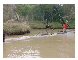
c). The lifting capacity of the loader is enough to handle extremely large trees. The largest one to date is a 36in diameter pine tree.
