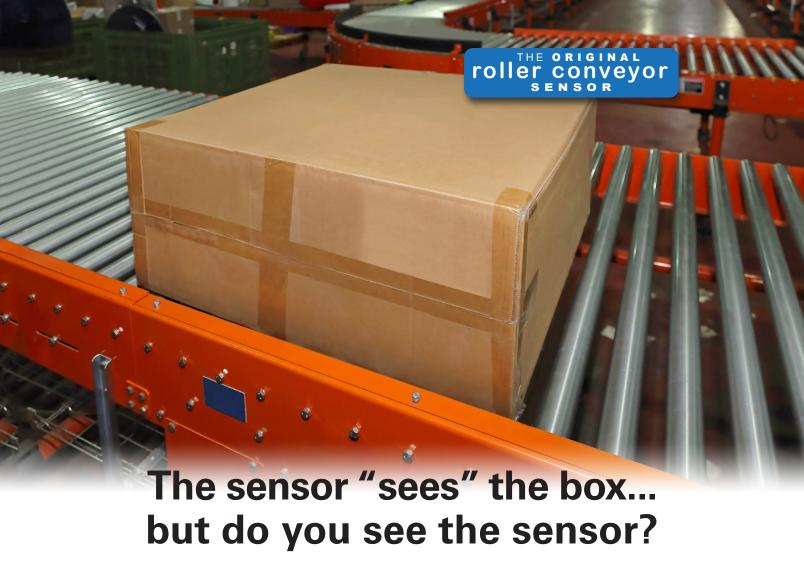
The sensor is there...you just can't see it. It's positioned right between the rollers underneath the box. By mounting the sensor between the rollers instead of on the side of the conveyor, you virtually eliminate the risk of sensor damage by items improperly positioned on the conveyor or next to the conveyor. And eliminating damaged sensors translates into a lot less machine downtime...
