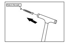
—Insert the wall anchors into the drilled holes and tap into place.
