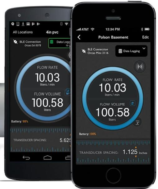
**Cypress** is a compact lightweight flowmeter with external power and communications for long-term flow monitoring. The Cypress Flowmeter connects with your mobile device via bluetooth or to the SoundWater Flow Computer. Either way, it works with your SCADA/PLC systems. It's a single piece ultrasonic flowmeter that installs on the outside of your pipe in a snap—and senses flow through the pipe wall.
