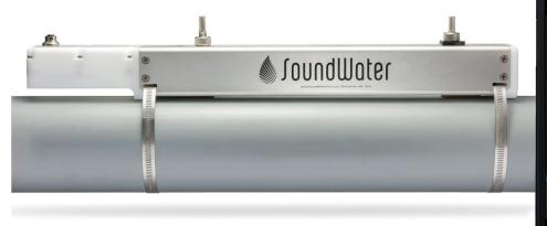
Cypress is a compact lightweight flowmeter with external power and communications for long-term flow monitoring. The Cypress Flowmeter connects with your mobile device via bluetooth or to the SoundWater Flow Computer. Either way, it works with your SCADA/PLC systems. It's a single piece ultrasonic flowmeter that installs on the outside of your pipe in a snap—and senses flow through the pipe wall.
