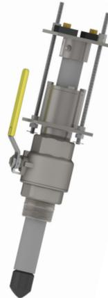
The SPI Mag Insertion Flow Meter provides a highly cost-effective solution for the accurate measurement of liquid flow in closed conduit, pressurized pipe applications. The SPI measures forward flow only and is suitable for line sizes from 2 to 96 inches. The SPI can be easily re-located to various line sizes.
