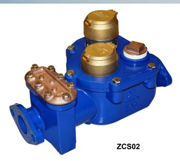
ate measuring device. Before the valve opens, all water flows through the low flow meter. As pressure rises the valve opens, allowing water to flow through both meters. Movement of the measuring elements are transmitted to drive magnets, which transmit the motion to driven magnets located within hermetically sealed registers. The magnets are connected to gear trains, which translate the rotations into volume totalization displayed on the register dial faces.
