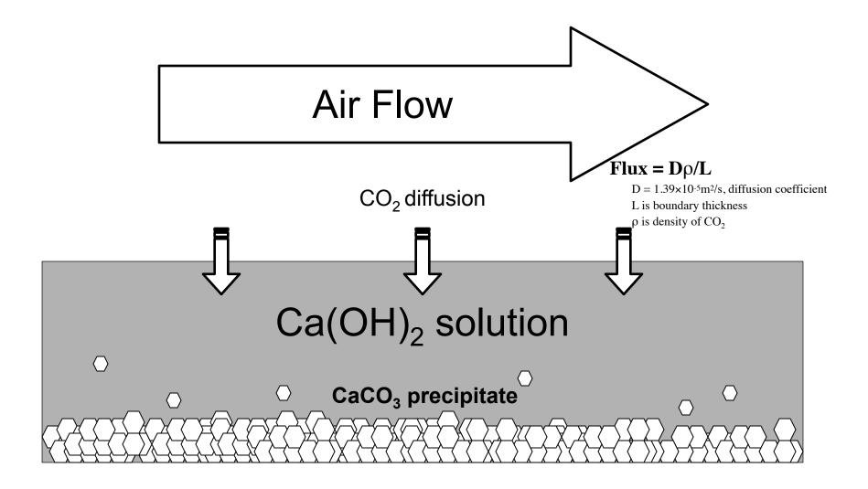
CO<sub>2</sub> mass transfer is limited by diffusion in air boundary layer
