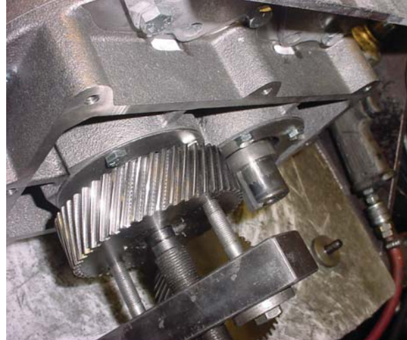
Figure 8-4 – Pulling Driven Gear with Bar Puller
