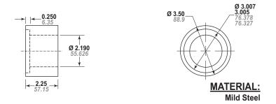
Figure 13-5 – Model 6000 Sleeve Pressing Ring (Use with Bearing Pressing Tool)
