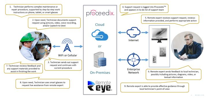
Figure Four: Combining digital work instructions and remote assistance capabilities
