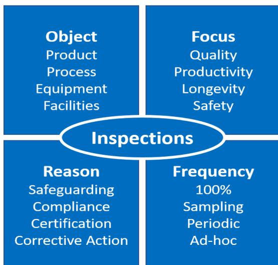
Figure 1: Manufacturing inspections
