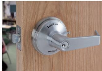
Until now, it required opening the door and checking the lever. PDQ's 135 LED Classroom Intruder function eliminates the need to open the door. Simply press the button on the lock, and...if the Red LED lights up, the outside lever is locked and secure. If the Red LED does not light up, this indicates the outside lever is not locked and secure.
