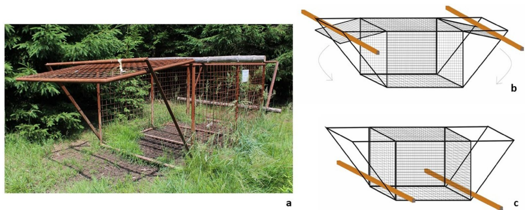
Figure 1. A box trap used for trapping wild boar at the study location (a). The open tipping door is secured by a wire. One end of the wire is attached to the door and the other end is hooked to the bottom of cage. The door is closed by manipulating the hook of the wire from inside the trap, usually during rooting. For a detailed photo of trigger mechanism, see Supplementary electronic material, SEM (Fig S1). Triggering the mechanism closes the door and releases the logs which secure the doors from the outside (b,c).
