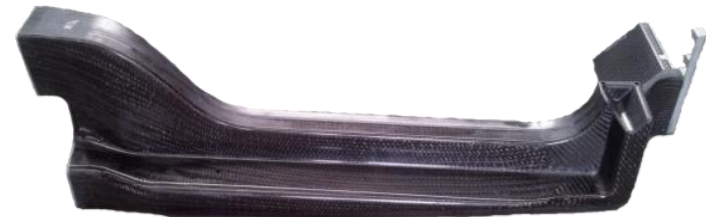
Preform Overbraiding Completed in 30 Minutes
