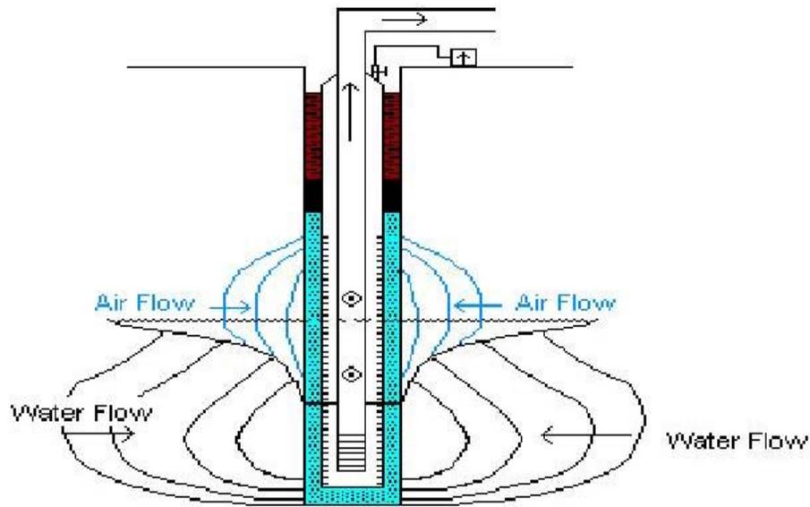
**Figure 1. Typical Bubblex<sup>SM</sup> Well Design:** Modified design of the extraction pipe and wellhead assembly facilitates lifting water in the vertical pipe, stripping volatile hydrocarbons and allowing monitoring for the several critical parameters such as annulus vacuum, water levels and collection of the water samples from the well and from the extraction pipe.
