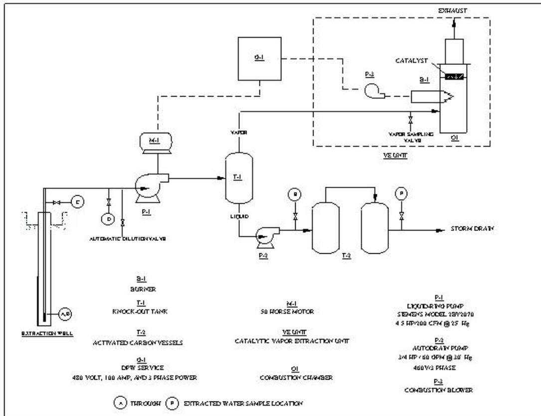
**Figure 3. Bubblex<sup>SM</sup> System Detail:** A, B, C, E, and F show the water sample locations where stripping test samples were collected.
