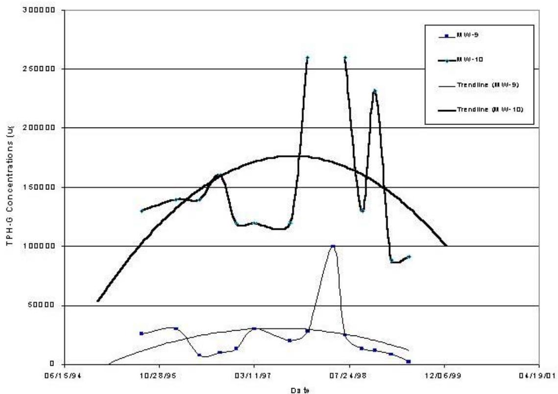
**Figure 6. TPH-G Concentrations in MW-9 and MW-10:** The increasing trend in concentrations is reversed after the system startup in April 1998.
