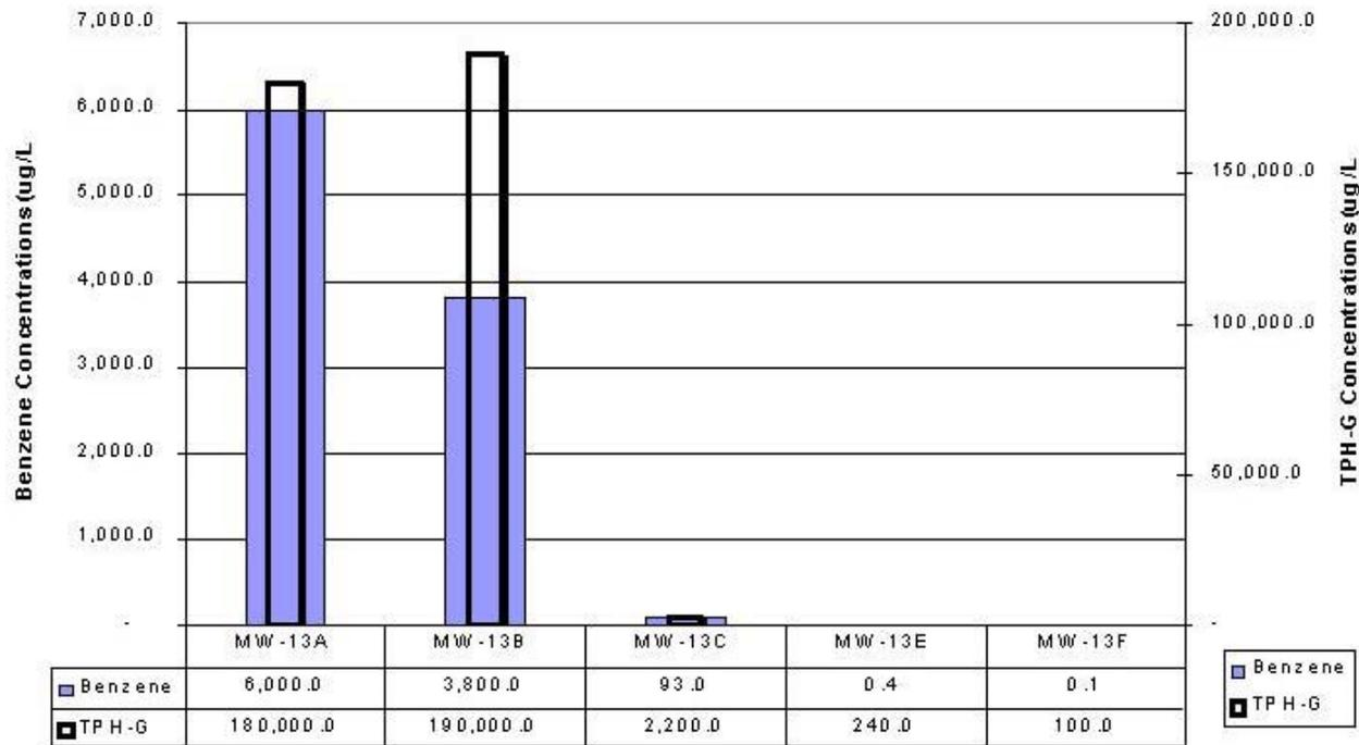
**Figure 4 Stripping test results (MW-13):** The concentrations of Benzene and TPH-G were reduced over 95% from the water table to the wellhead (from B to C) due to stripping in the Bubblex<sup>SM</sup> extraction pipe. Additional 95 to 98 % stripping occurred in the pipe between the wellhead and AC unit (from C to E).
