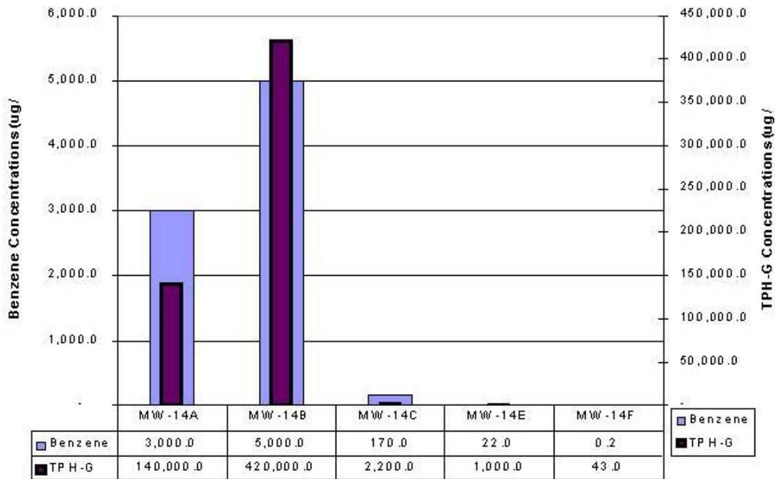
**Figure 5 Stripping test results (MW-14):** The concentrations of Benzene and TPH-G were reduced over 95% from the water table to the wellhead (from B to C) due to stripping in the Bubblex<sup>SM</sup> extraction pipe. Additional 95 to 98 % stripping occurred in the pipe between the wellhead and AC unit (from C to E).
