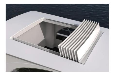
Once rotated to the venting position, the louvres can be fully retracted to give an open area. Alternatively, leaving the louvres vented allows a free-flow breeze and dappled shade.
