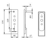
Assembly kit for glass thickness max 12 mm. **FOR CENTRAL LOCK ASSEMBLY TYPE TOUCH BAR CAN BE USED WITH EXTERNAL CONTROL FOR DOOR OPENING.** PVD finish cover plates, gaskets, fixing screws. Instructions.
