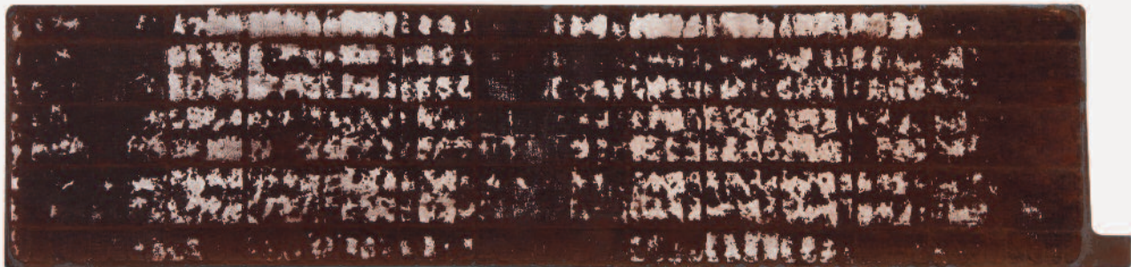
Competitor's plate formed in the battery case. White areas indicate plate is not fully formed.
