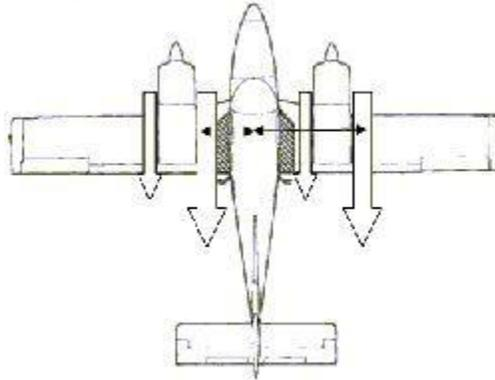
This is basically the equal and opposite reaction of p-factor. If the left engine fails, the effect of the p-factor creates more induced flow farther away from the longitudinal axis of the aircraft creating a rolling moment.
