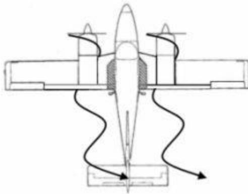
This spiraling air from the left propeller, due to its direction of spiral, hits the rudder creating more airflow to make the rudder more effective. If the left engine fails, the spiraling slipstream from the right engine spirals away from the rudder.
