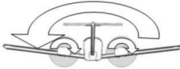
Torque tries to roll the airplane opposite of the propeller's direction of rotation. If the left engine fails, torque tries to roll the aircraft to the left, making it more difficult to **raise the dead** engine.
