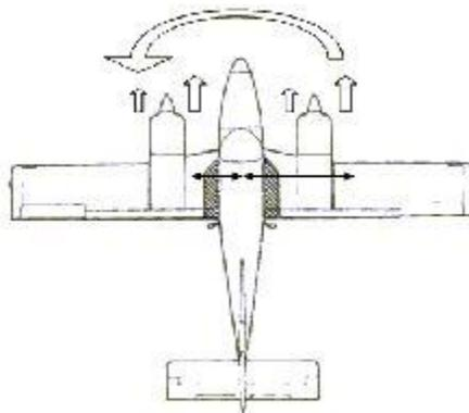
If the left engine fails, the p-factor being produced from the right engine is farther from the longitudinal axis of the aircraft, creating more of a yawing moment.
