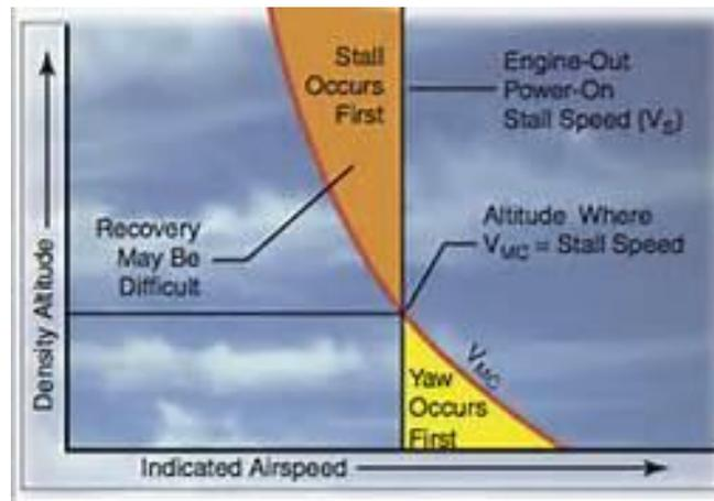
If both Vmc and stall speed are reached at the same time, a spin is almost inevitable.
