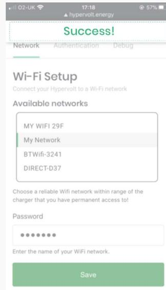
After you hit Save once, the charger will disconnect from your phone and try to connect to the network you have selected. It will do so irrespective of your password being valid or not. The LED ring around the unit will also switch to the same colour as the front LED display. If however the network connection is unsuccessful, within 1 minute the charger will revert to a **WHITE** LED ring around the unit and you can retry the setup process.
