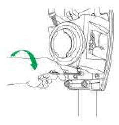
e. Disconnect the connectors from the right side of the controller.
