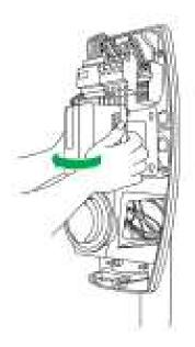
h. Tighten the clamps with a socket wrench to secure the charging station on the Combi pole.
