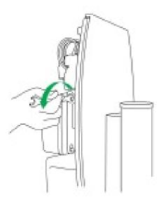
g. Remove the controller up to release the bolts from the slotted holes in the bracket. Move the controller to one side to access the Combi pole clamps.
