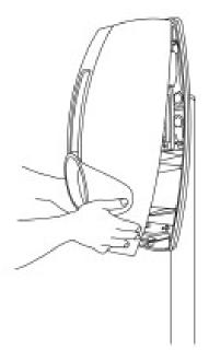
f. Tighten the bolts at the bottom of the cover using the 5 mm hex key (supplied). When the charging station is mounted on a wall bracket, the space to tighten the cover bolts is very small. Use a small socket wrench with a 5 mm hex key bit, or short Hex Ball Key.
