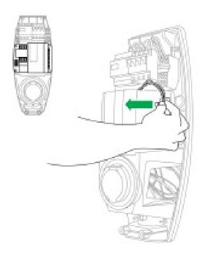
f. Loosen but do not remove the bolts attaching the controller to the bracket.
