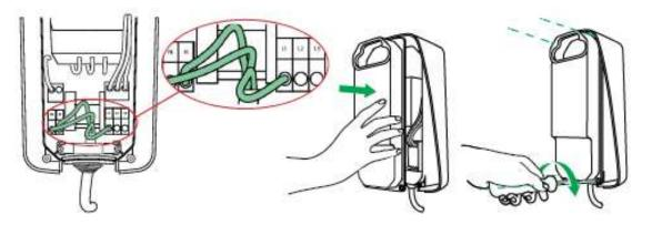
Note: Installation example of a 1-phase connection of Elvi.
