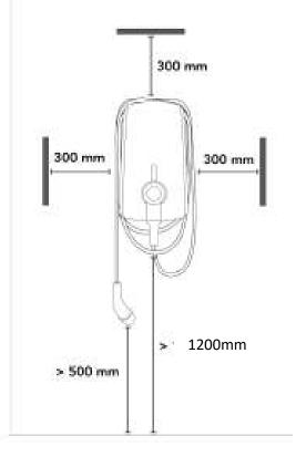
**Note:** The above illustration indicates a recommended standard installation height. Observe and comply with the local accessibility regulations.
