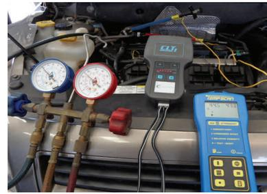
In the illustrations above, in the left picture, the compressor is not activated, (although the front drive plate of the compressor is turning) and the pressures are almost equal. In the right picture, the CLT control unit has the compressor swash plate at the full angle. Unfortunately many technicians see the left picture results and assume the compressor is bad causing them to replace the compressor unnecessarily. This often results in a failed repair and a compressor returned to the supplier.
