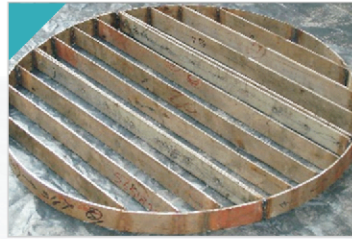
Column internals (supports plate/ distributor, and collector)
