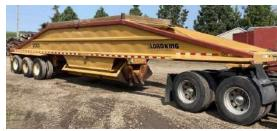
1994 Load King Belly Dump Model 2060: 43', tri-axle, grease banks, air ride suspension
