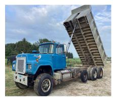
1986 Mack RS688L ST 8x4 Dump Truck: Mack 300 engine, air lift pusher axle, Maxitorque 7 speed trans, camel back suspension, 181,290 miles, 17' aluminum dump box
