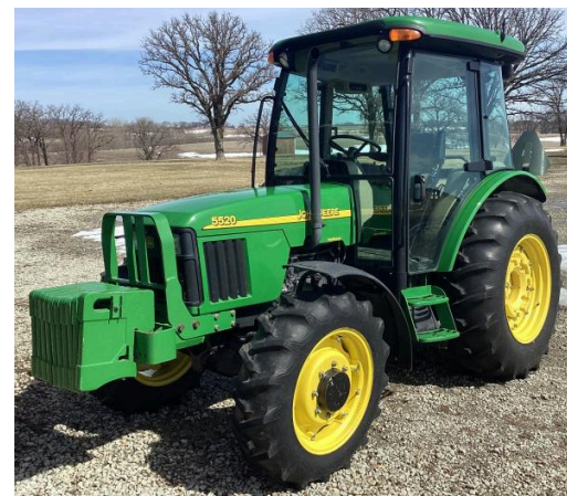
John Deere 5520 Utility Tractor, 89hp, Diesel, Power Reverser, 4wd, Front Fender, 3pt, Full Cab Heat, Air, Radio, 540pto, 2 Sets Hyd Rear Remotes, Front Weight Pack, Rear Wheel Weights, 729 Hrs, (1 Owner)
