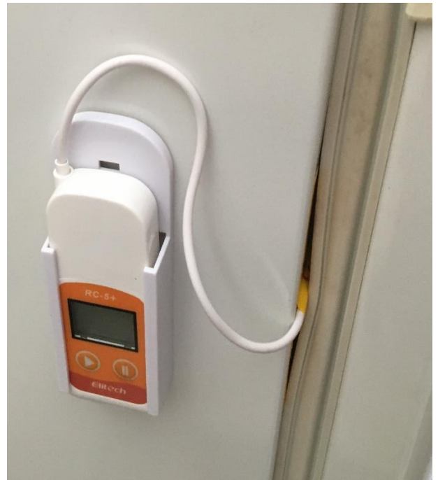
Datalogger on fridge
