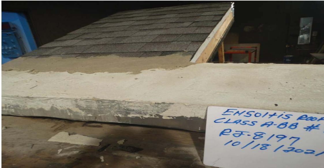
Photograph 1: Ensoltis Above Roof Deck Thermal Insulation System. Owens Corning Sure Nail Shingles test deck assembly from the top.
