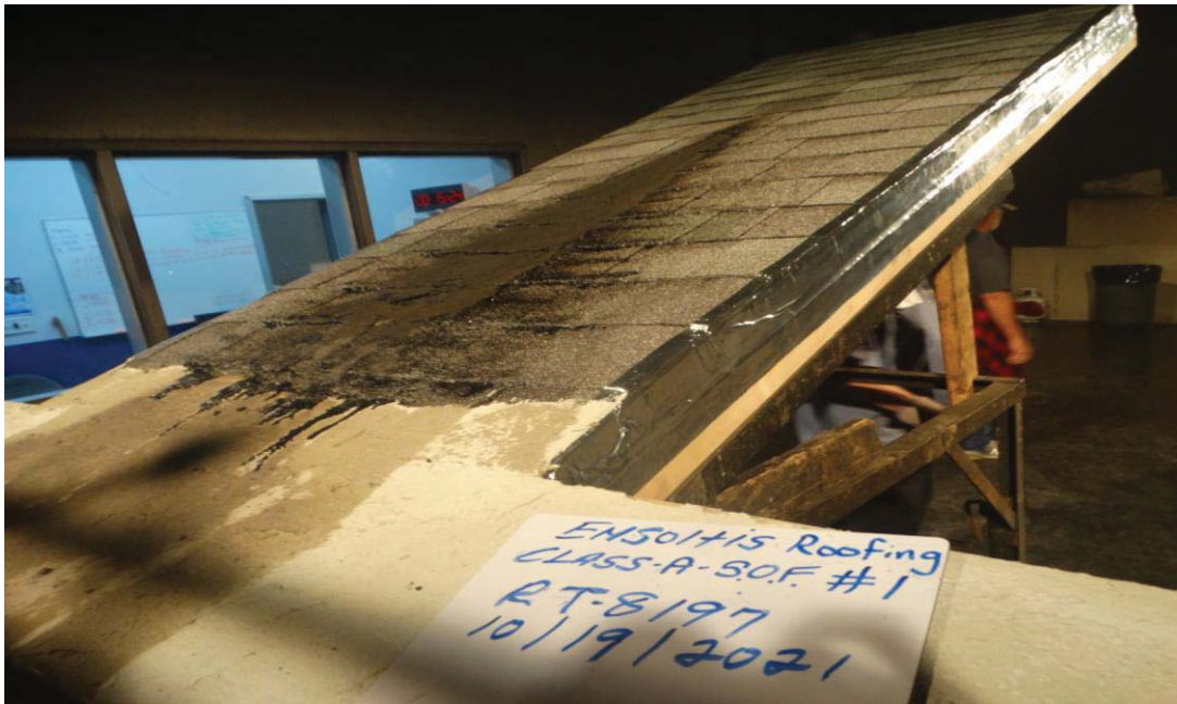
Photograph 12: Class A Spread of Flame test deck assembly from the top.
