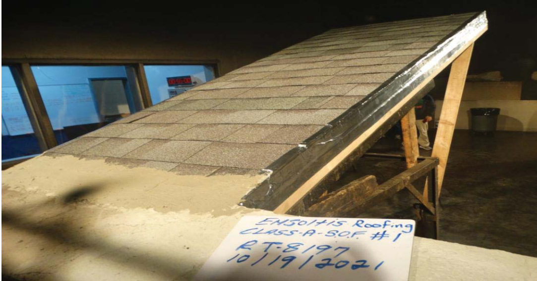
Photograph 11: Spread of Flame test deck #1 Owens Corning Sure Nail Shingles test deck assembly from the top.
