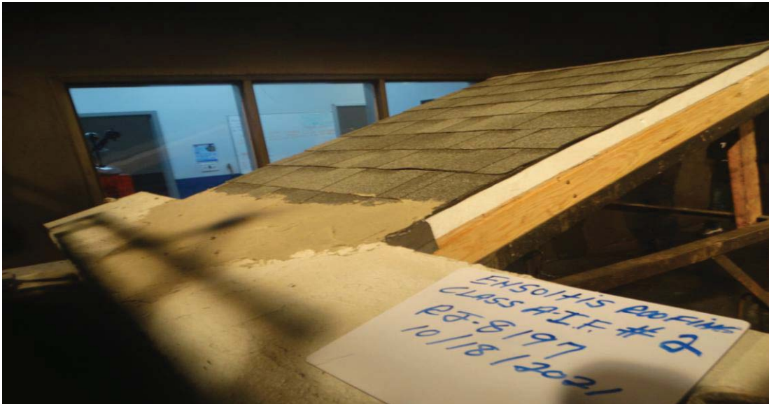
Photograph 9: Intermittant Flame test deck #1 Owens Corning Sure Nail Shingles test deck assembly from the top.
