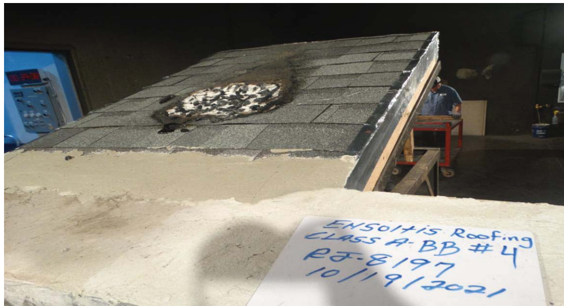
Photograph 8: Class A Burning Brand test deck assembly #4 from the top.
