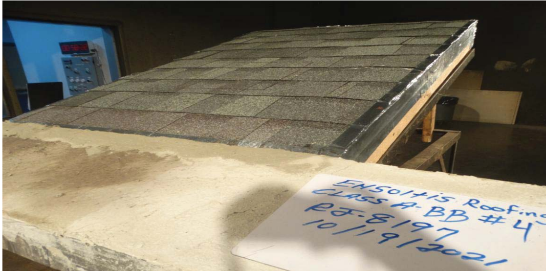
Photograph 7: Ensoltis Above Roof Deck Thermal Insulation System. Owens Corning Sure Nail Shingles test deck assembly from the top.
