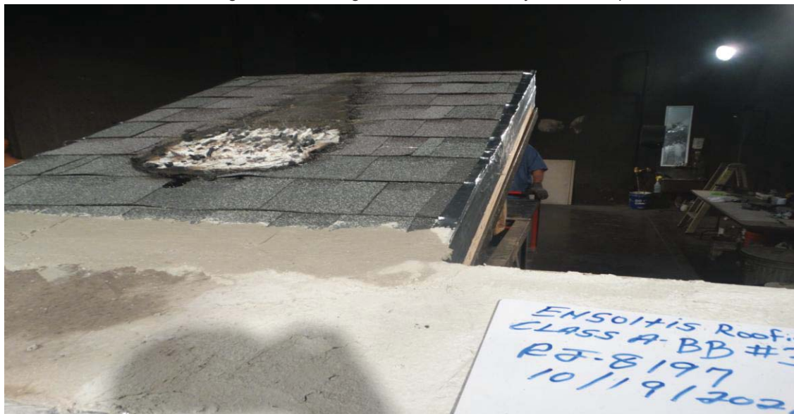
Photograph 6: Class A Burning Brand test deck assembly #3 from the top.
