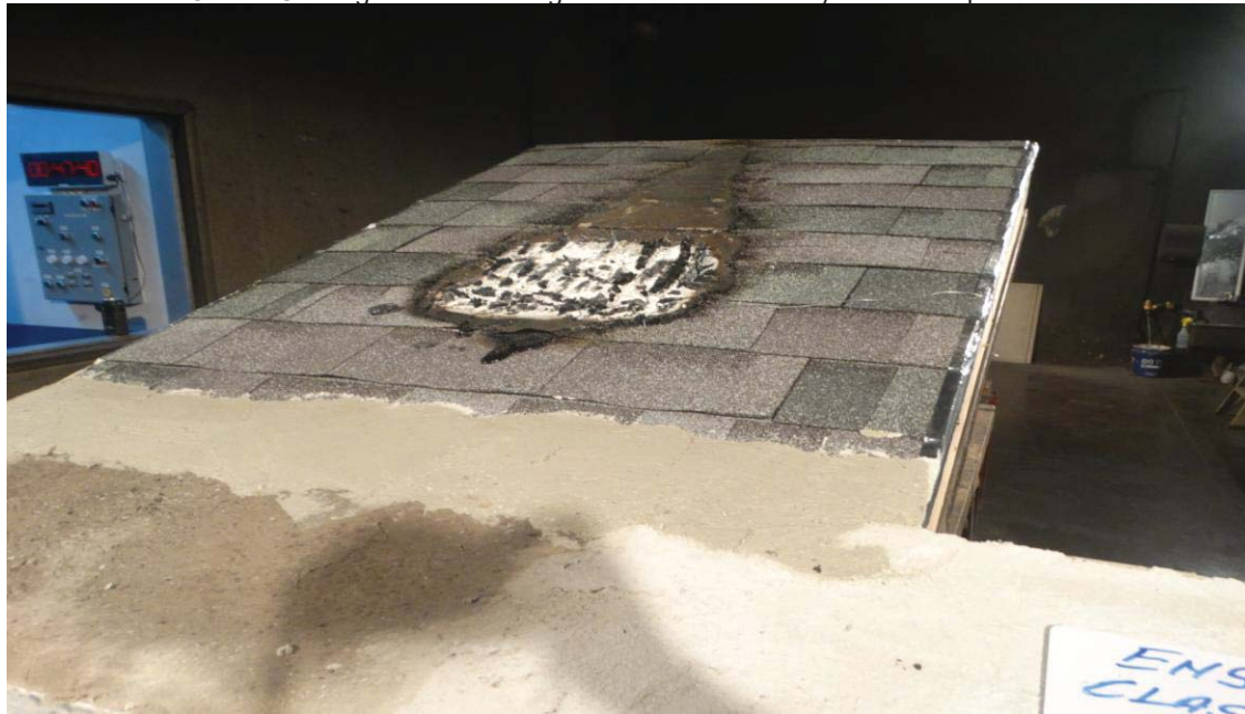
Photograph 4: Class A Burning Brand test deck assembly #2 from the top.
