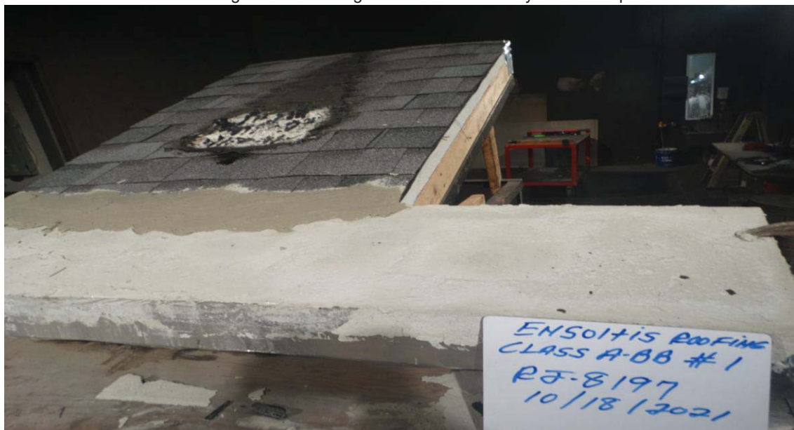
Photograph 2: Class A Burning Brand test deck assembly #1 from the top.
