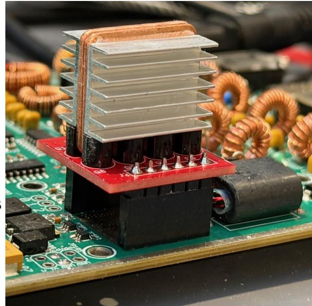
3. Insert the 2 male headers on the underside of the red supplied PCB and solder one pin only on each one on the top side of the board.
