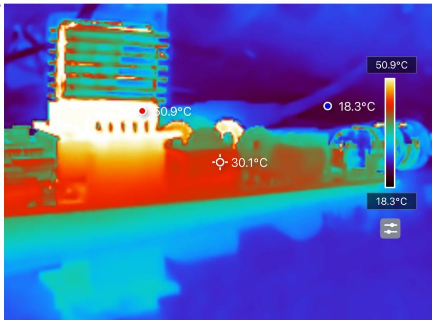
This was at the end of a 15 second TX period in FT8. I typically saw the finals run between 65C and 70C at the end. They would then cool down to around 50C (shown above). The cycle would repeat.
