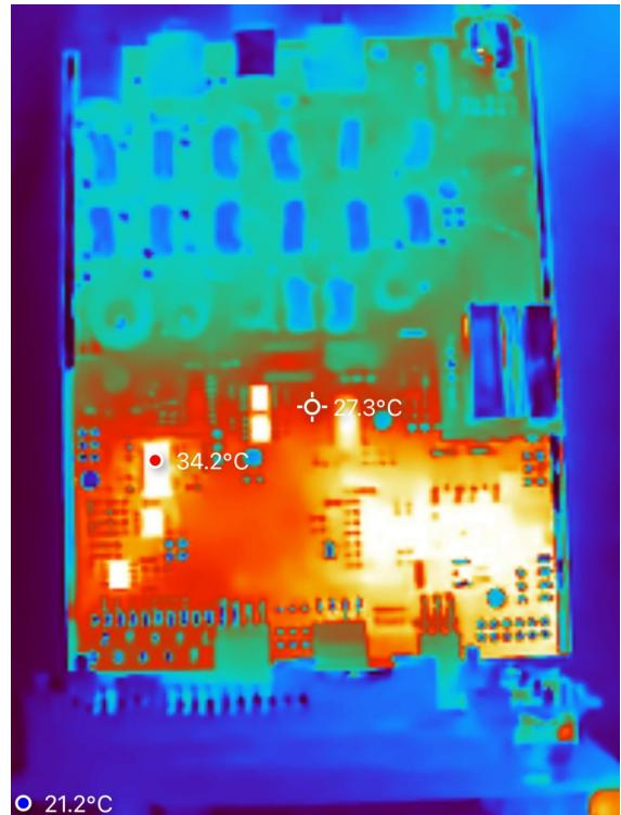
This is the same shot after about 5 seconds of transmission. You can clearly see the 10 meter LPF components - L517, L518, :522, D5129, D520 & C536 getting warm. The LPF toroid reached 41.3C after 5 seconds. Also of note is the 8x finals board getting hot. The copper portion of the heat sink is thermally connected to the board.
