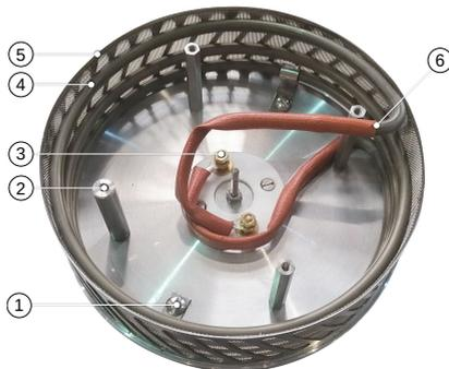
Figure 8: Head disassembling step 3
