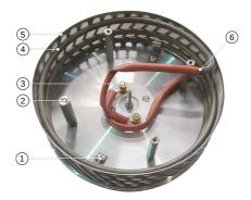
Figure 8: Head disassembling step 3
