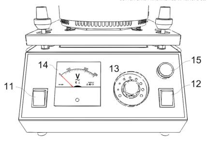
The front panel has the following controls: Switch (11) turns on the electric motor which rotates the spinning head; Switch (12) turns on the heating element; Adjustment Knob (13) regulates power to the heating element and thus controls its temperature; Voltmeter (14) indicates actual voltage supplied to the heating element.
