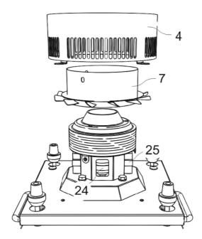
To replace brush units (25) first remove the screws securing the brush unit. Remove the unit carefully and inspect the carbon brushes. If the brushes are worn more than half of the length, they should be replaced.
