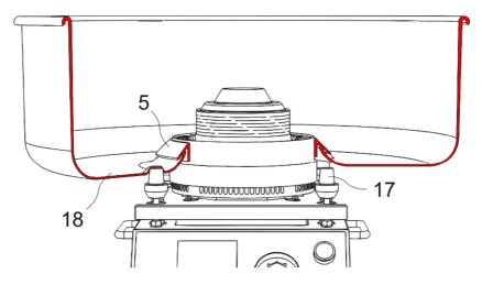
Floss pan indentations (shown above) should fit rubber support legs (17). carefully install silicone collar (5) on the stator with the collar edge overlapping the pan.
