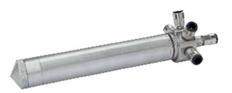
One of the reasons for the reproducibility of the Lab 1 Glass Laboratory Spray Dryer is the durable and precise nozzle technology. The nozzle comes with a de blocker needle which can be pushed through the nozzle in case of clogging. The de blocker frequency is user selectable. Optional, nozzle cooling is available. The nozzle can be cooled with regular tap water. Spraying of heat sensitive product is possible.
