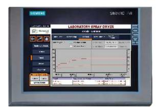
A data trend screen shows a record of the air temperatures, heater output and feed liquid pump output during the experiment. The user can visually see the temperature record and quickly understand it.
