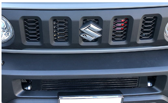
Standard Kit - Intercooler is visible behind the bumper in the traditional position.
