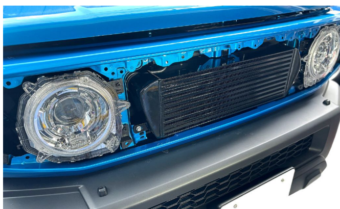
Hi-Mount Kit - Intercooler is higher up behind the grille for a stealth look.
